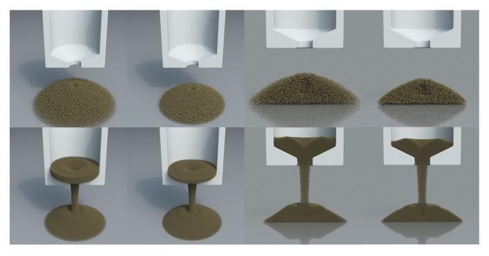
Fig. 9. **Pouring sand**. The top row depicts the result of an explicit simulation with a coarser grid size ( $dx = 10^{-2}$ ), while the bottom row corresponds to a finer grid size ( $dx = 10^{-3}$ ). The first and third column correspond to a projection step without volume correction, while the second and fourth column uses our volume correction algorithm.
